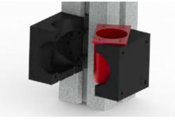
Figure 112 Design of the hinges including all components, making rotations and replacement of components possible
