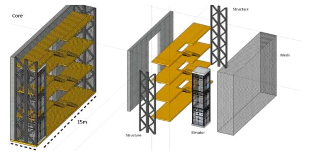
Figure 15 Exploded view core
