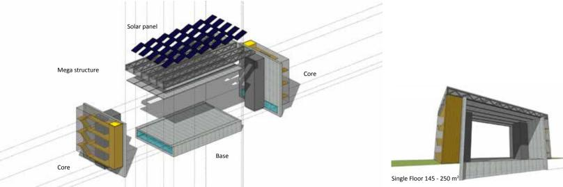
Figure 16 Isometric perspective
