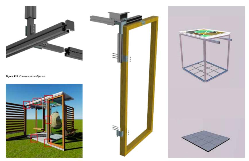
Figure 138 Connection wooden frame - steel frame
