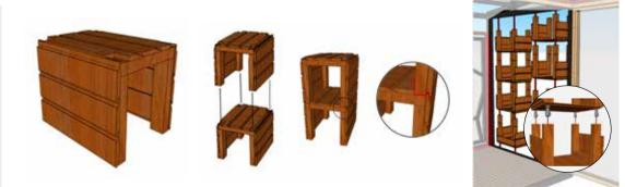
Figure 115 Creating a complete interior from existing wooden panels and beams based on boxes linked to each other or used separately
