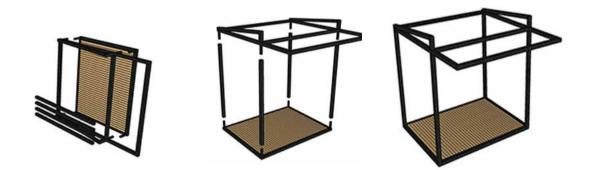
Figure 107 Building up the main frame
