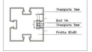
Figure 113 Detail steel frame
