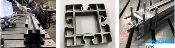
Figure 17: Manufacturing of the GTB LAB metal profile (P1)
