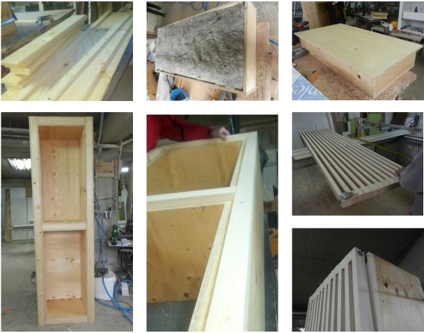
Figure 24: Manufacturing of the GDC facade module
