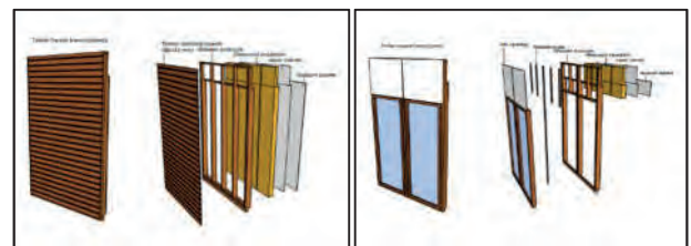
Figure 4: Open and Closed wooden frames
