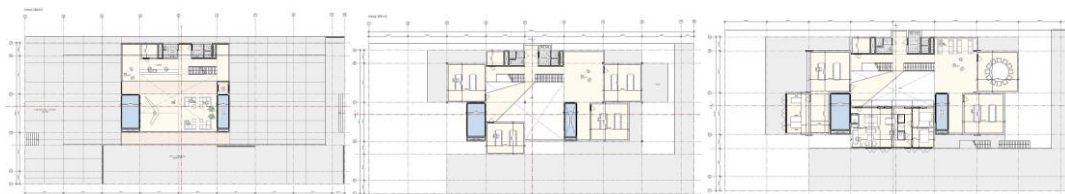
Figure 3: Position of the core elements that is not restricting number of use options,
